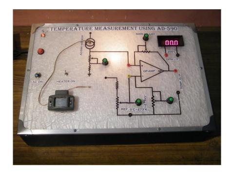
This is AD-590 Temperature sensor based one of sensor study kit. Details circuit function, adjustment & calibration procedure we have incorporated in this kit. Op-Amp based circuit & actual circuit diagram is given in manual. Mini heater also inbuilt. This kit consist of:-
